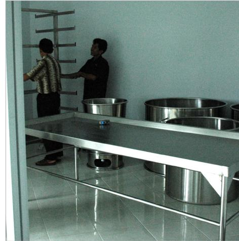
A model factory demonstrates environmentally friendly and hygienic tempe production including stainless steel drums and replacing firewood with gas.
